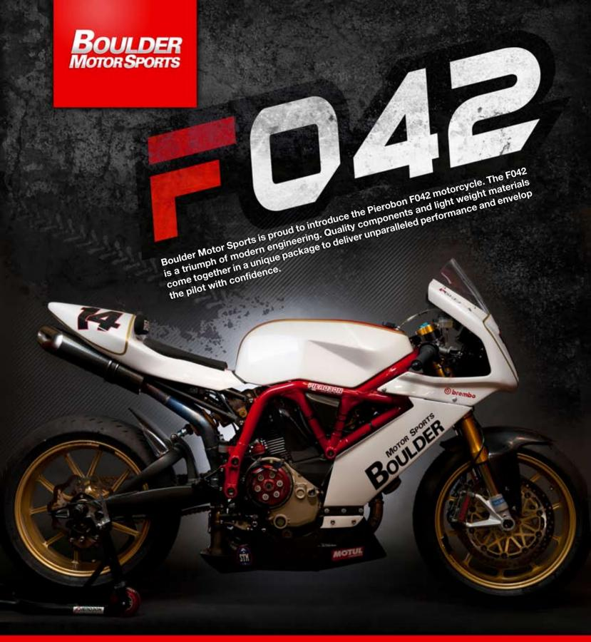
rame: Tubular aluminum using some billet components
